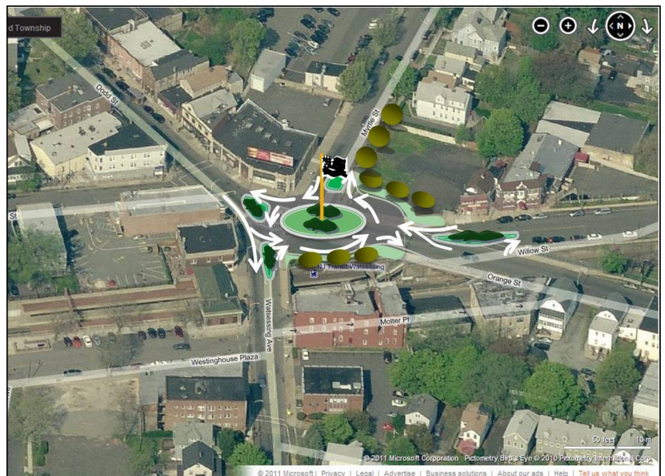
Figure 19: Sketch of roundabout at "5-Point" intersection to regulate traffic flow and provide safety islands for pedestrian crossings, as well as a landscaped foreground for the historic train station.
